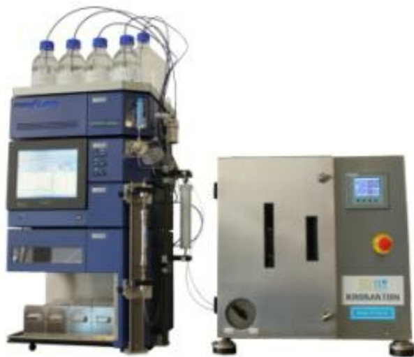
FCPC A with automatic fraction collection system and software package, 50- 1,000 ml
