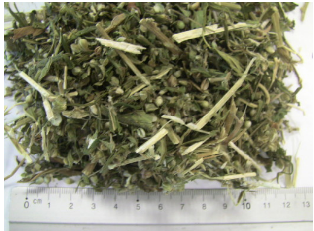
Picture 4: Industrial hemp after pre-cutting in SM 400; 20 mm sieve
