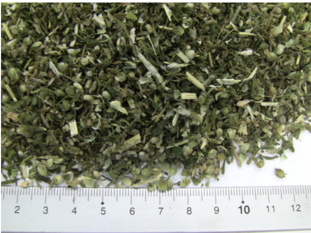
Picture 3: Industrial hemp after pre-cutting in SM 400; 6 mm sieve
