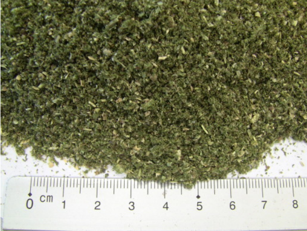
Picture 5: Industrial hemp after fine-grinding in SM 300
